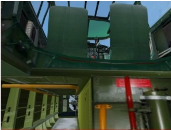
This graphic is taken from the Mid-Atlantic Air Museum flight simulator of their B-25 aircraft, Briefing Time. Note the two pilot and co-pilot chairs on the flight deck and the bombardier's tunnel at the lower left.
